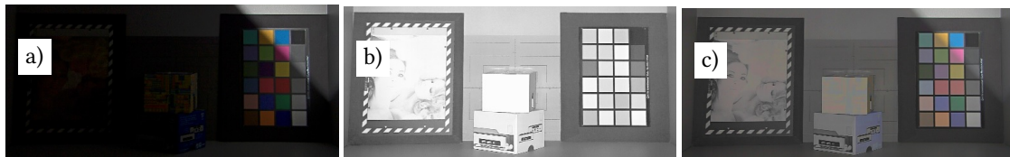
Figure 1.2: Concept of the image merge algorithm: color image (a) and grayscale image (b) are digitally combined into a superior merged image (c).
