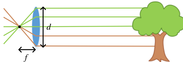
Figure 2.2: A convex lens of diameter d focuses parallel light to the focal point. The distance between the lens and the focal point is called the focal length f .
