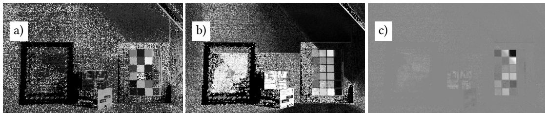
Figure 3.5: Hue (a), saturation (b) and visibility (c) channels in the HSV color space.
