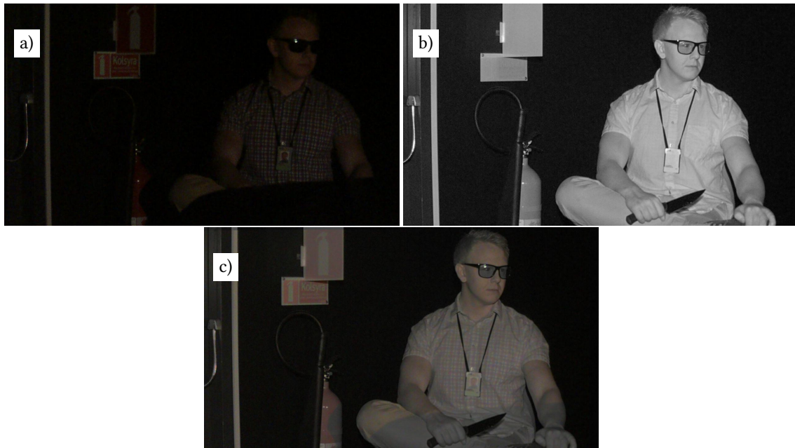
Figure 4.8: Test scene of a human holding a knife. Color image (a), grayscale image (b) and merged image (c).
