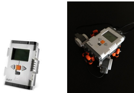
Figure 3: (left) NXT brick CPU [3], (right) Omni wheels mounted on the NXT [4]
