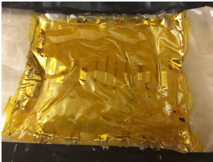
Figure 16 – Finished gold foil strain gauges. In order to establish a connection, wiring was attached onto the substrate using silver epoxy glue.
