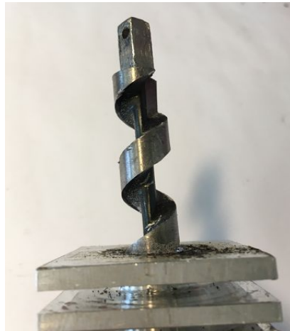
Figure 9.1 Auger stuck in extruder
