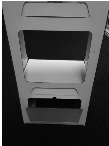
Figure 11.20 Cutout for easily removal of hot air and hatch for power supplies
