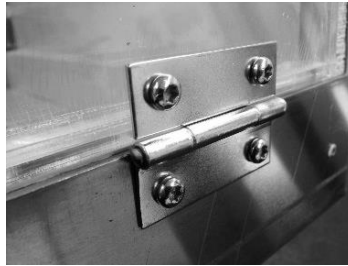
Figure 11.15 Hinges used for attaching the lid to the aluminum casing
