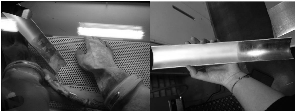
Figure 11.2 Sand blasting of bars
