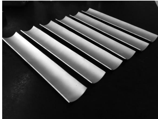
Figure 11.3 All six bars after sand blasting
