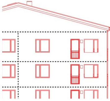
Figure 7 Facade with Fire Barriers
