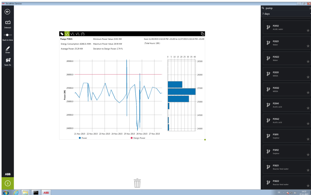
Figure 23 – Energy monitor of the pump
