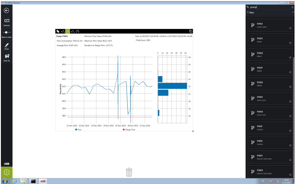
Figure 24 - Flow monitor of the pump
