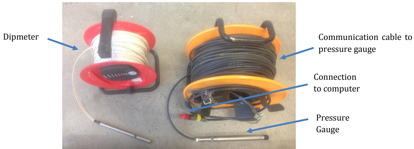
Figure 3-2 Dipmeter (left) and pressure gauge communication cable, pressure gauge and where the cable is connected to the computer (right). Photo: Sofia Hallerbäck
