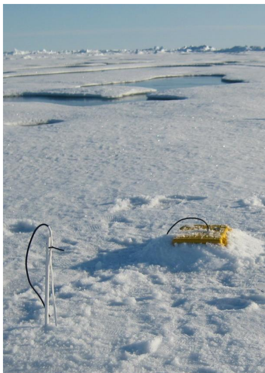
Figure 7. A deployed IMB buoy on the Arctic sea ice. The buoy consists of a long chain of sensors (one the left hand side in the picture), one every 2 cm, with the ability to measure the temperature profile down through the snow and ice layers. The sensor chain is connected by a cable to a logging controller and a battery power source in an enclosure (yellow in picture) stationed on the ice surface (Dybkjær, 2015).
