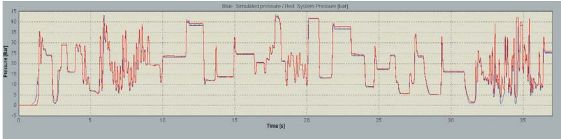
Figure 4.16 Pressure measurements. Measured pressure (red) and simulated pressure (blue).
