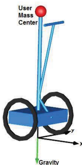
Figure 5.1 Two-wheeled self-balancing vehicle 3D model visualization in Dymola
