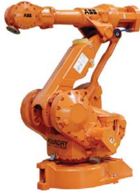
Figure 2.2: ABB IRB 4400, an example of ABB serial robot.
