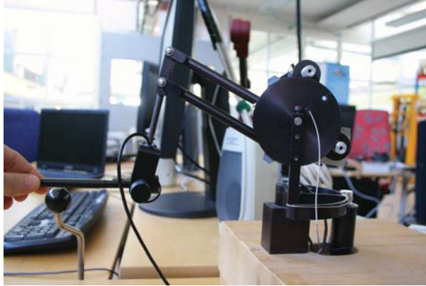
Figure 6.5: Haptic device at the startup. In order to increase the operative workspace, the Phantom has to be initialized with this position.
