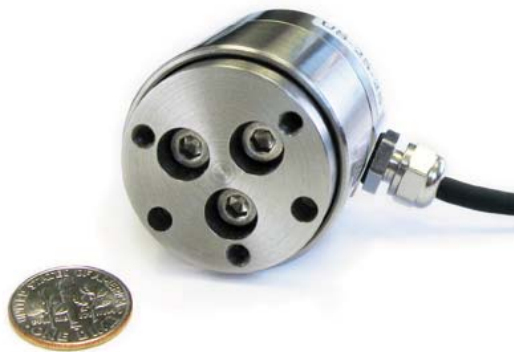
Figure 12: The ATI nano25 force sensor used in experiments.
