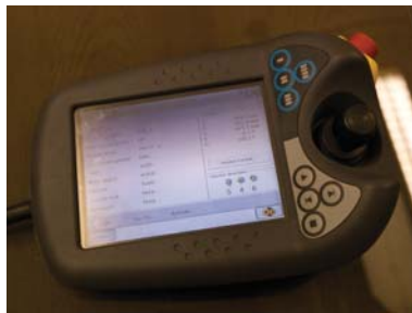
Figure 14: The FlexPendant can be used to jog the robot or execute RAPID based programs
