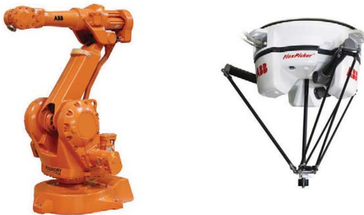
Figure 1: Left: a ABB IRB 2400, a typical serial robot. Right: The ABB IRB 360 FlexPicker, based on parallel structure[1]
