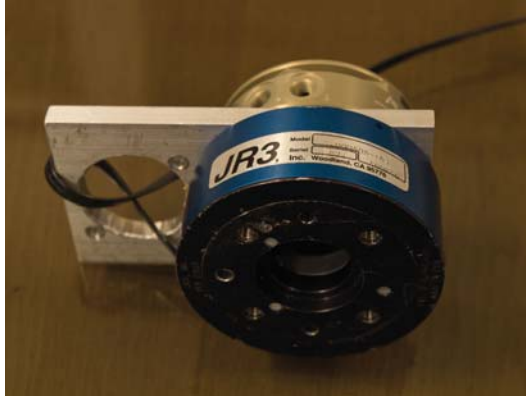
Figure 11: One of the two JR3 force sensors used in experiments. The force sensor is attached to a mounting plate that allows mounting on the robot.
