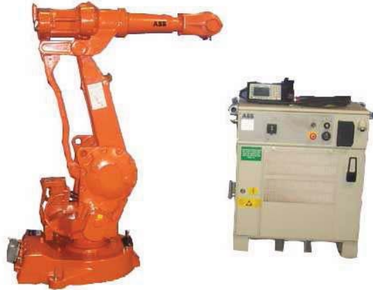
Figure 2: IRB 2400-16 and S4CPlus control cabinet with the Teach Pendant produced by ABB
