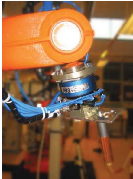
Figure 4: JR3 force sensor with the tool holder attached to the wrist of the IRB 2400-16 in the Robotic Lab
