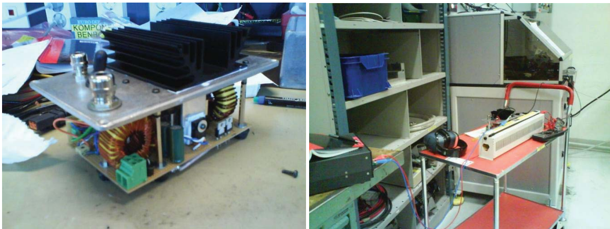
Figure 12.1 To the left the demo DC/DC converter is shown and to the right the DC/DC converter together with the alternator rig is shown.
