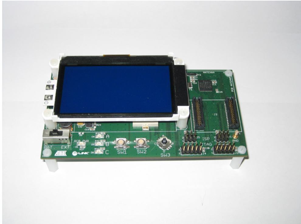
Figure 4.11 Photo of the LCD module in the eZeeNet kit.
