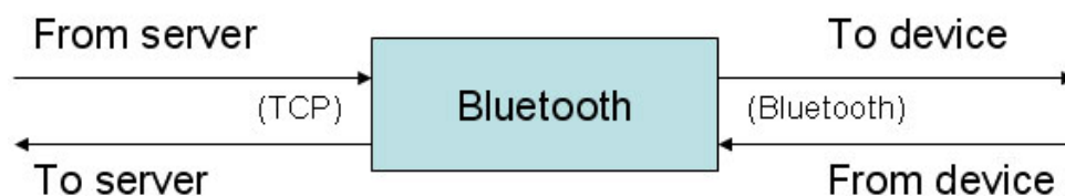
Figure 4.7 Schematic overview of a Bluetooth communication protocol module
