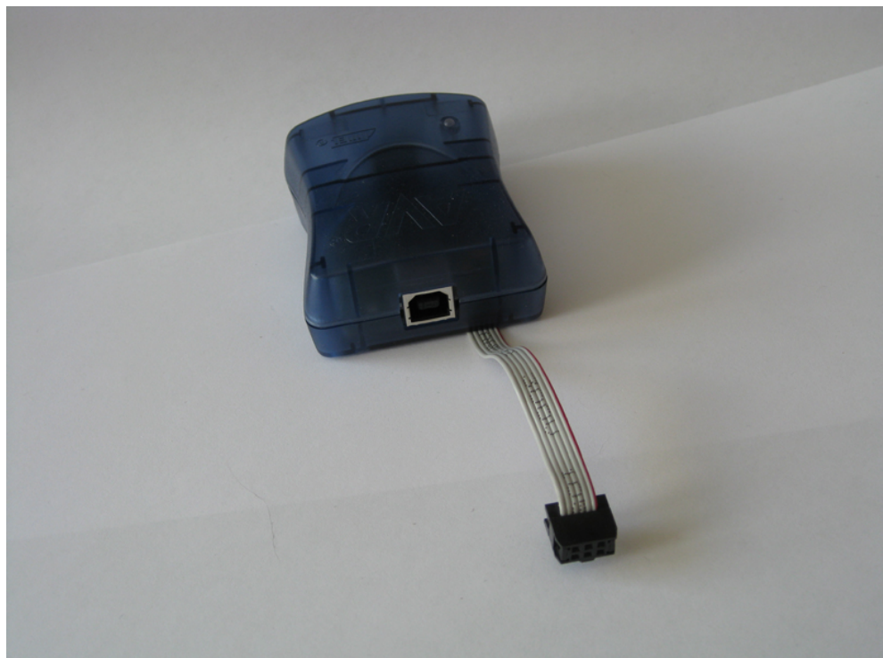
Figure 4.12 Photo of the AVRISP mkII used to program the AVR1281 microcontrollers in the eZeeNet ZigBee kit.
