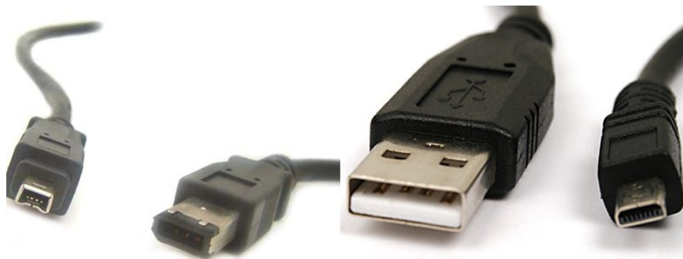
Figure 2.1 FireWire connectors to the left and USB connectors to the right.
