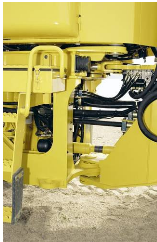
Figure 2: Picture of the steering pivot point between the front and rear axis.
