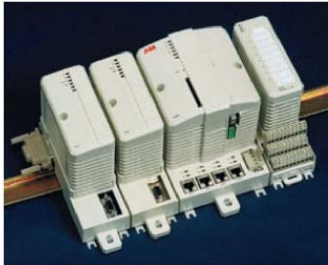
Figure 2.1: A process module on a rail accompanying other modules.
