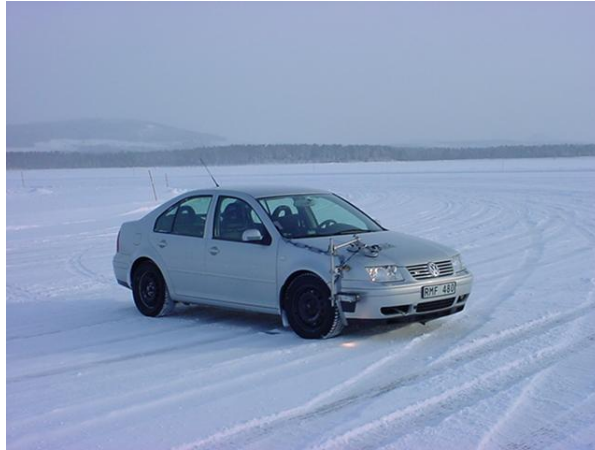
Figure 4.3 – Test vehicle equipped with an optical sensor
