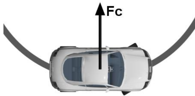
Figure 2.4 – The centripetal force at a turn
