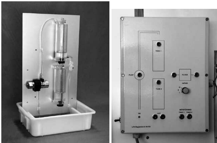
Figure 4.1: The tank process consisting of two tanks with a small hole in the bottom. The water is pumped into the upper tank and then flows down into the lower tank, then out of the process.
