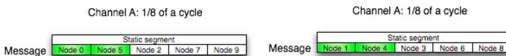
Figure 32 – Shows the different cycles used for the distributed nodes. Note that the order of the slots is changed so the sending nodes are in the beginning of the cycle.
