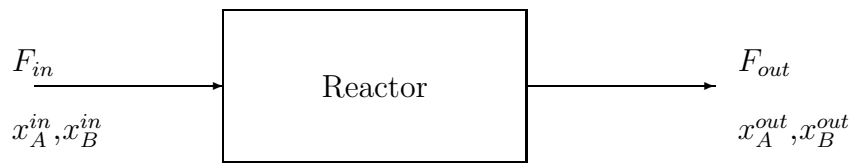
Figure 2.2: Constant volume reactor
