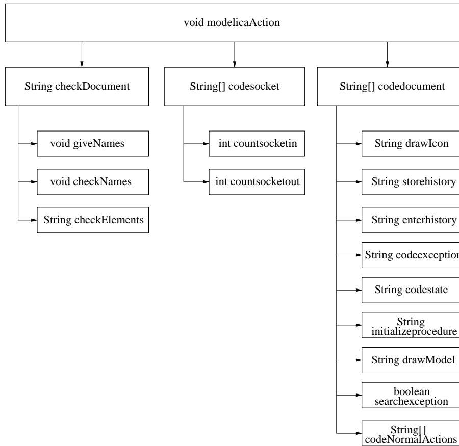
Figure 4.1: Function structure of the code generator
