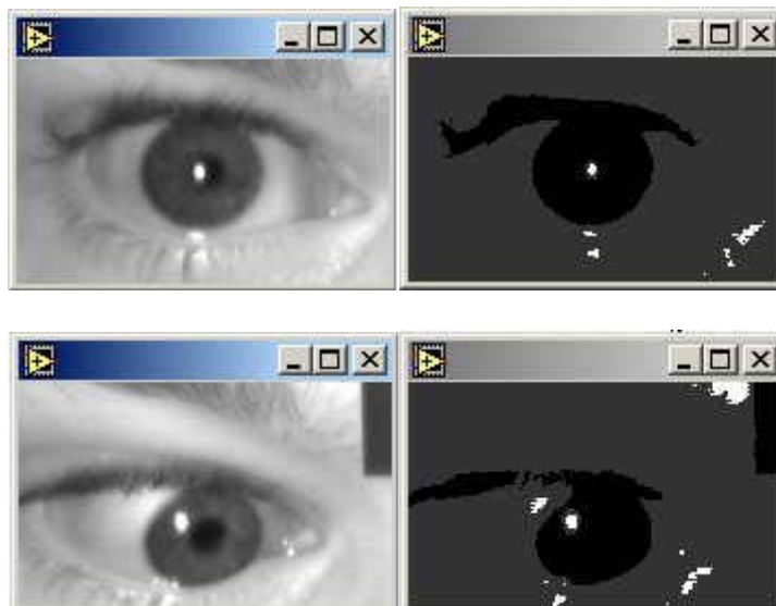
Figure 25. Images of the same eye taken from the same test sequence. 2 threshold levels were applied. (100 and 240)
