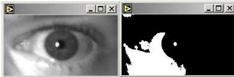
Figure 24. Binary Thresholding. Left, the original image. Right, the binary image. (Threshold level 170)
