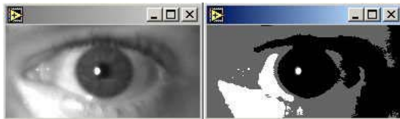
Figure 23. Thresholding. Left, the original image. Right, the image after thresholding. Two threshold levels were employed. (100 and 200)
