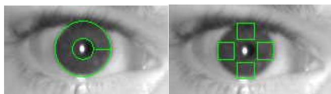
Figure 27. Left, the iris is selected. Right, it is split into four regions to determine the light intensity for the threshold levels
