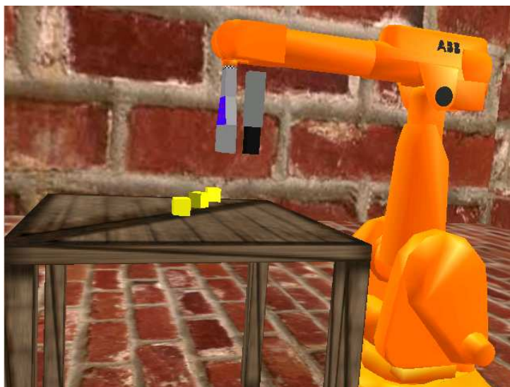
Figure 2.4: The "Virtual Robot". Here, the IRB 2000 has been set up for interaction with small dice lying on a table. The scene is observed by three cameras, one attached to the end-effector and two cameras in a stereo configuration in front of the robot (not shown in the Figure)
