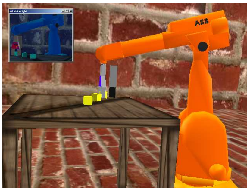
Figure 4.2: The robot is grasping the rear dice. This position was achieved using a single-camera setup. In the upper left of the image, a camera image after image processing is depicted. The detected feature points are marked.
