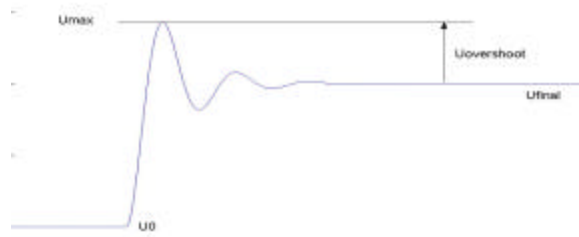
Figure 12: Control signal with overshoot.
