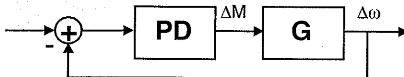
Figure 3.1: Controller structure for PD-controller
