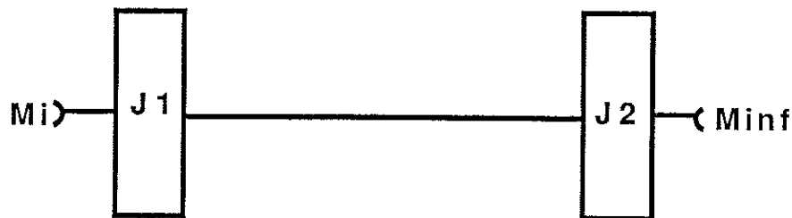
Figure 4.1. A simple rigid body model of a robot axis.
