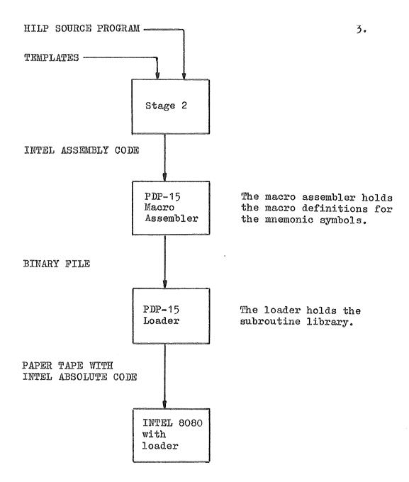
fig 1. From HILP 80 source to loaded INTEL 8080.
