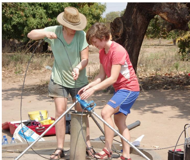
Figure 30 Adjusting the tripod-pulley (blue upper part). Photo by Torleif Dahlin.
