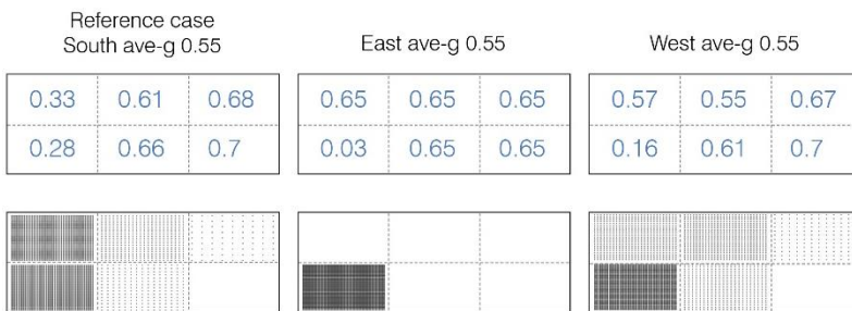
Figure 53: Ray tracing module output of re-distributed g -value and uniform frit pattern for south- (Reference Case), east- and west-oriented cases.
