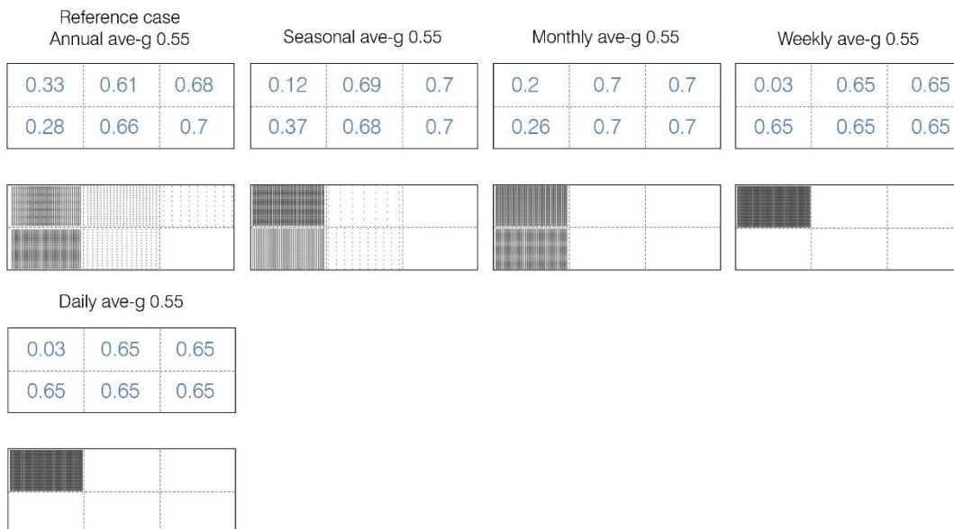
Figure 61: Ray tracing module output of re-distributed g -value and uniform frit pattern for the cases with annual (Reference Case), seasonal (summer), monthly (August), weekly (3.-9. August) and daily (2.August) analysis period.
