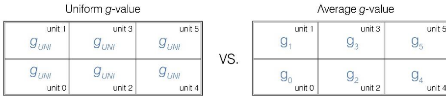
Figure 29: Glazed facade with uniform g-value and average g-value, for which results were obtained and are presented in the Section 6 Results.
