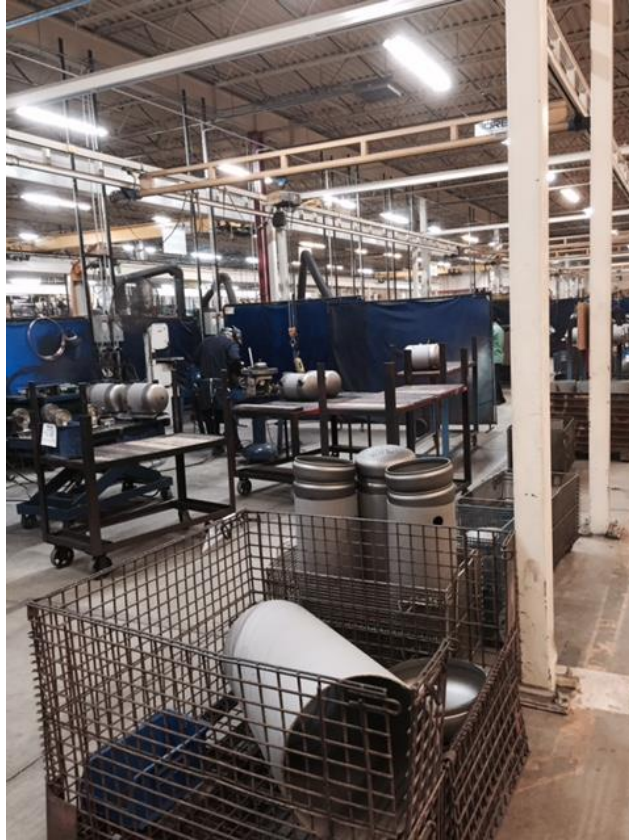
Figure 24: A view of some of the different material carriers in SU small. The image displays both baskets with kitted orders and carts with WIP.
