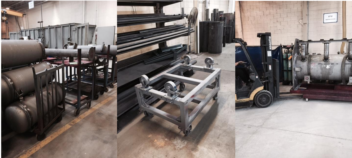
Figure 25: A view of three different material carriers. From the left; small carts for small vessels, cart meant for large pipes or relatively large vessels and at last customized pallet with wheels meant for really large vessels.
