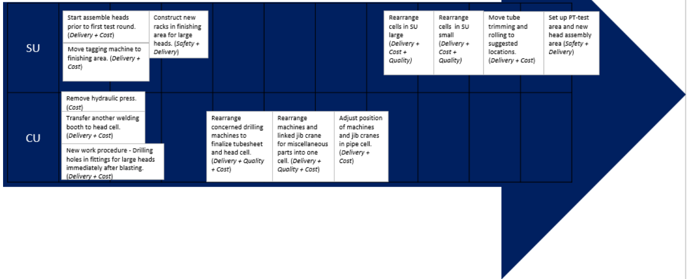
Figure 40: An example of the sequence the long term proposals can be implemented in. Key performance indexes that are affected positively by each activity are included in parenthesis in each text box.
