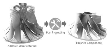
AM is a process where a part is built additively, often in a layerwise fashion. This allows for complex shapes, with some AM limitations.
