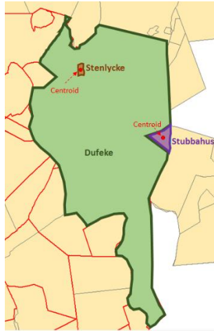
Figure 4.12: Initial Property Unit “Stenlycke” has its centroid located within another initial property unit “Dufeke” in Halmstad parish
