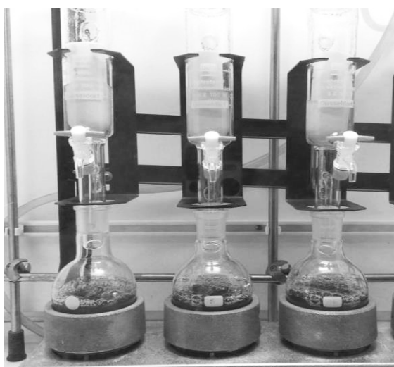
Figure 4. The extraction set-up with Soxhlet apparatus where the sample is put into the thimbles (white, filter paper tubes) and extracted into the receiving flasks at the bottom.
