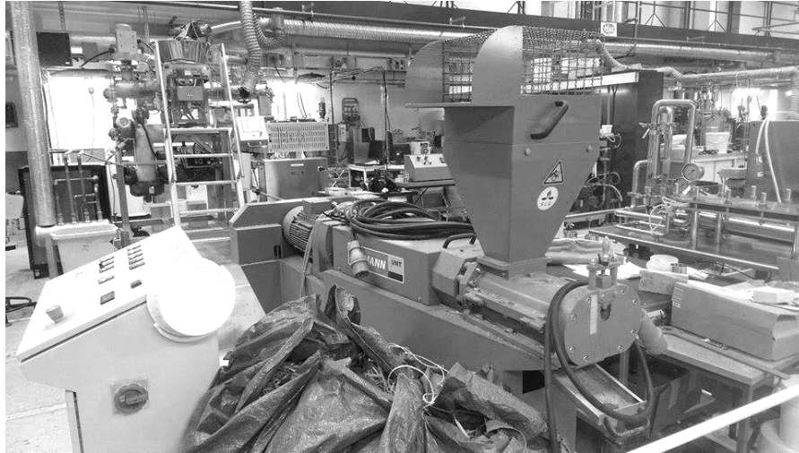
Figure 2. The twin screw extruder used in this project where the input is on top of the machine and the outlet opening can be seen to the right in the picture.
