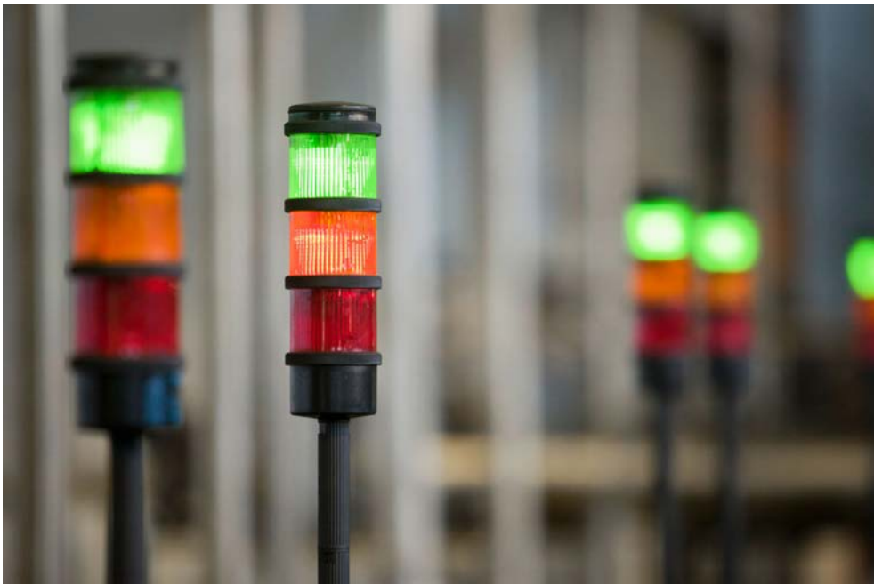
Figure 17 Andon lights (Welotec, 2016).
