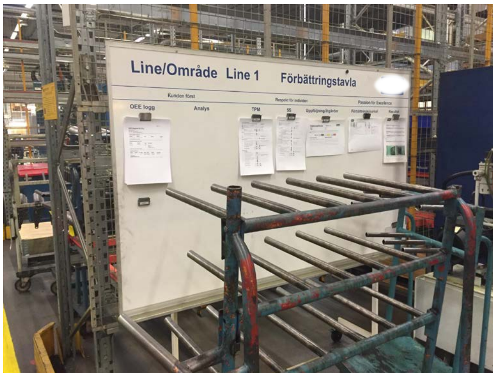
Figure 36 Lean status board blocked by rack indicating low priority of Lean (Carlsson & Fröberg, 2015).
