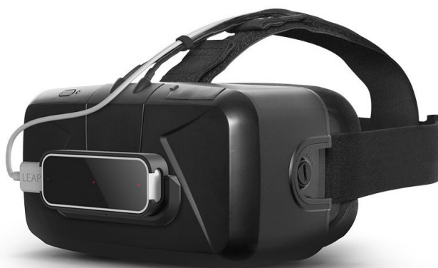
Figure 2.3: The Leap Motion mounted on an Oculus Rift DK2 (Development Kit 2)
