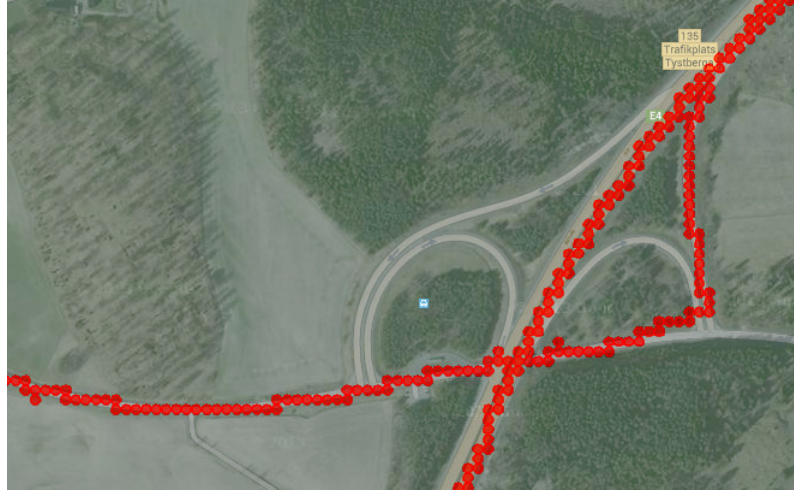
Figure 3.5: The same map portion created from a single trace, with Bresenham interpolation. Map data: Google, Lantmäteriet/Metria.
