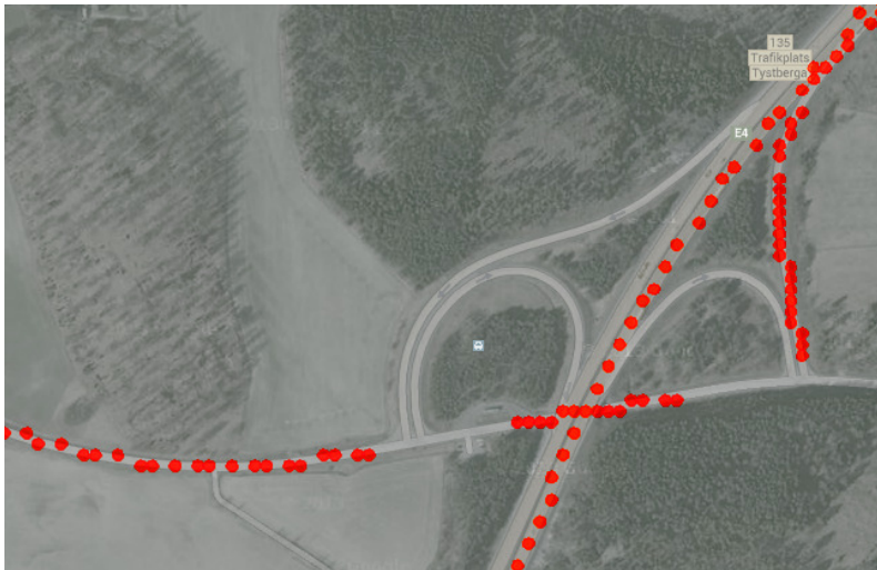
Figure 3.4: A piece of a map constructed using each discrete GPS sample only. Map data: Google, Lantmäteriet/Metria.
