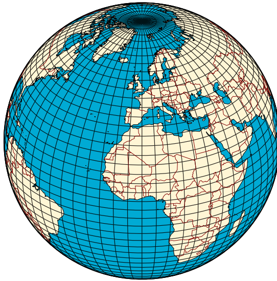
Figure 2.1: The earth divided into quadrilateral pieces as defined by equally spaced WGS84 coordinates. Image: Hellerick on Wikipedia. Creative Commons Attribution-Share Alike 3.0 Unported license.
