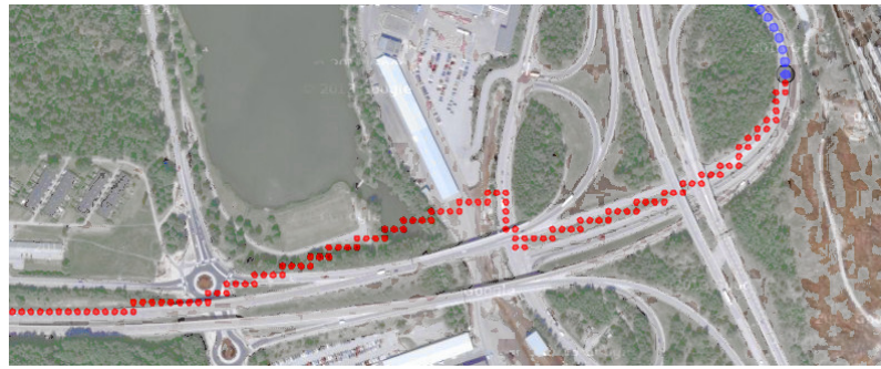
Figure 4.11: Erratic behavior of directional algorithm in a select situation. Map data: Google, Lantmäteriet/Metria.
