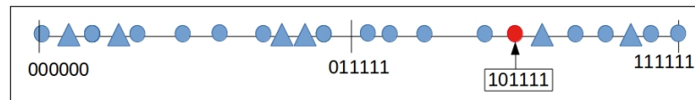
Figure 2.1: A graphical representation of the identifier space in Kademlia. Circles represent nodes and triangles represent resources.
