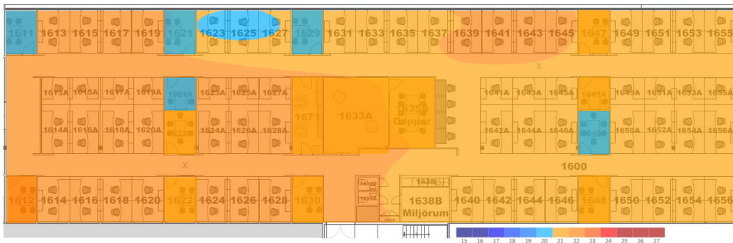
Figure 7.2: Heat map within the pilot facility showing different temperature at different areas within the Ericsson facility. The figure is taken as a snap-shot from the web based visualisations tool Energidirigenten pilot .
