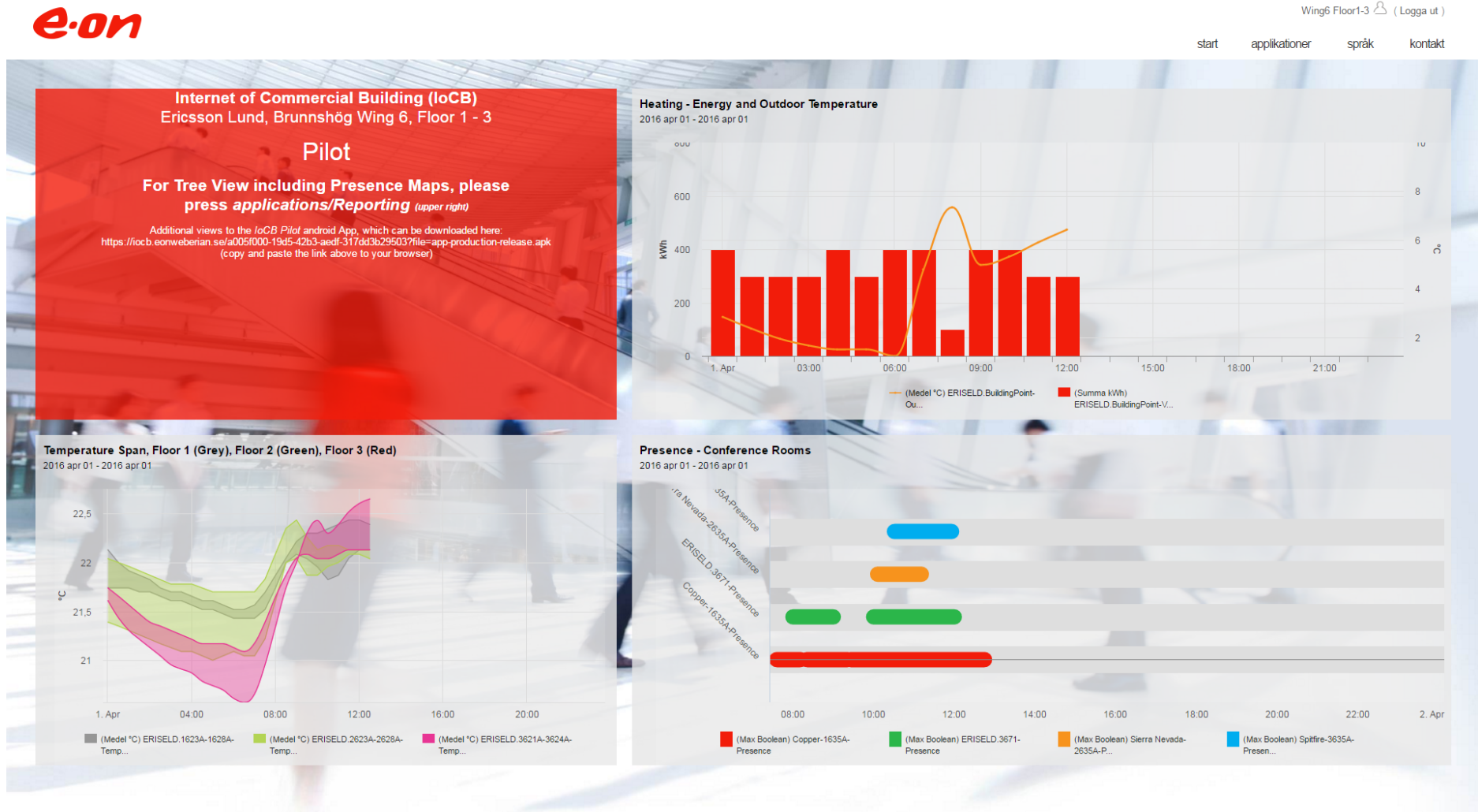
Figure 6.2: The web dashboard interface for Energidirigenten pilot. The view includes some initial information regarding the pilot project and some visualisations of energy flows and presence. The graphical profile follows the existing interface of Energidirigenten developed by E.ON.
