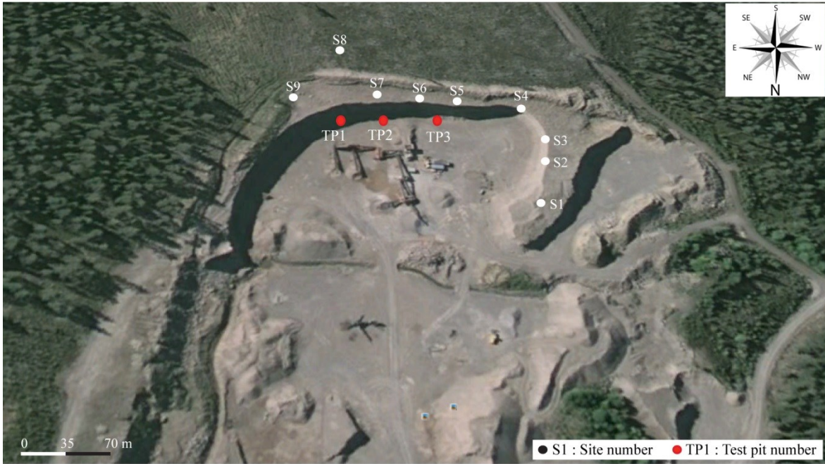
Fig. 4. Google Earth overview crop of the Fiskarheden pit and position of described sections are marked by white dots numbered S1-S9. Test pits in front of the main section wall are numbered TP1-3 and marked with red dots.
