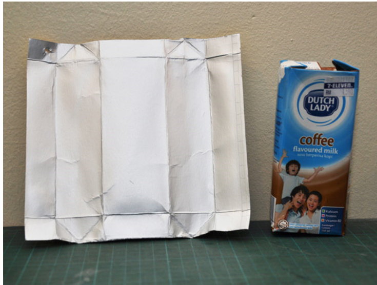
These Figur 1 Picture of creased Tetra Pak paperboard [13]
