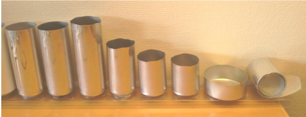
Figure 1.3. The cup (second from the right) is transformed in the bodymaker. The most left can is the resulting product.
