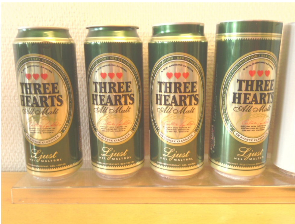
Figure 1.4. Labelled cans before and after necking.
