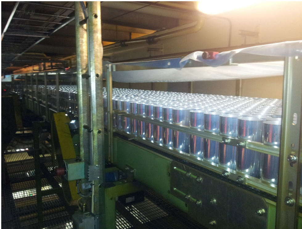
Figure 1.6. Conveyor belt acting as accumulation buffer.
