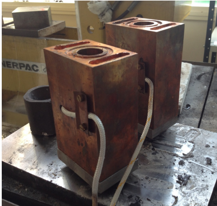
Figure 7: The copper mold used to change the cooling rate.
