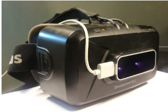
Figure 4.4: Oculus Rift DK2 and Leap Motion integration.
