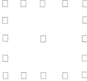
Figure 6: The set of surrounding pixels for the LBP feature \text{LPB}_{16,2} , each pixel with the distance of \text{sup}(l, k) = 2 from middle
