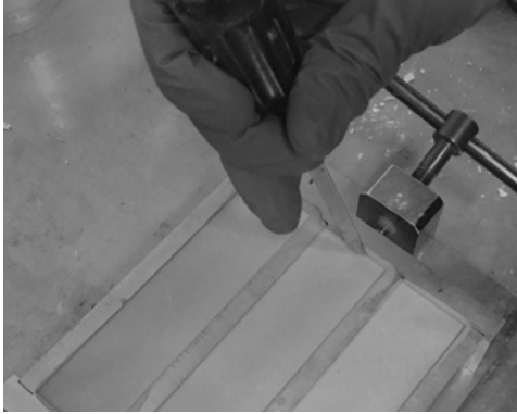
Figure 13 – Extraction of prisms from the mould.
