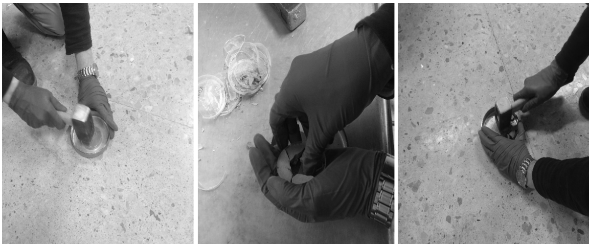
Figure 12 – From left to right: the procedure for extracting SLCs from plastic Petri dishes
