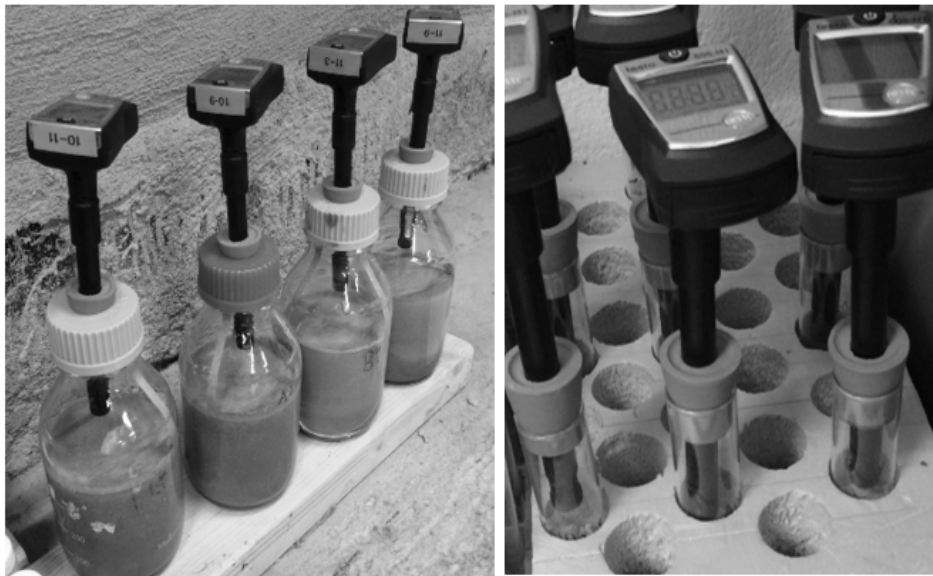
Figure 25 – 500 ml vials and test tubes with attached RH-sensors
