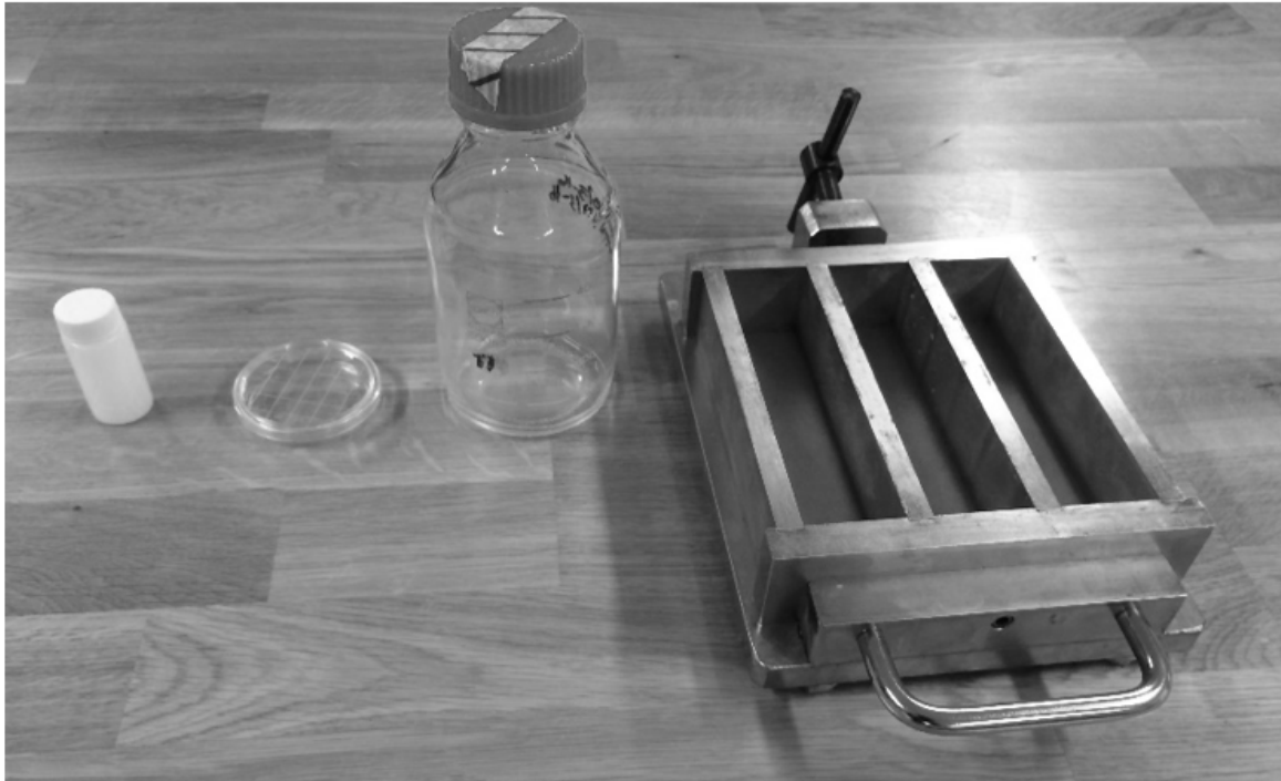
Figure 8 - From left to right: 20 ml PE vials, plastic Petri dish, 500 ml vial and a mould for prisms.
