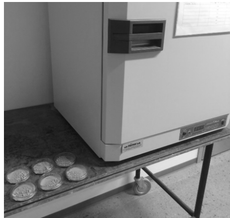
Figure 16 - Samples cooling after 24 hours in drying oven
