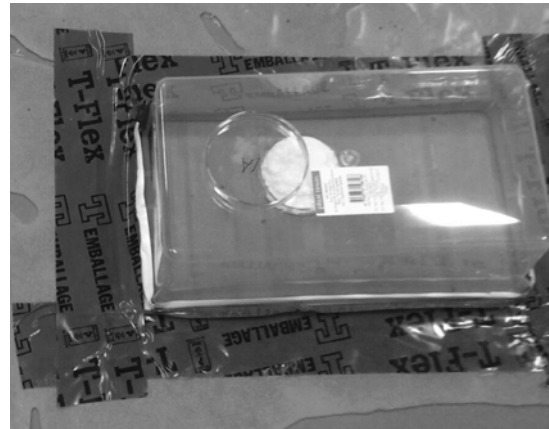
Figure 4 – Dry calcium chloride placed under a dome-shaped hood.
