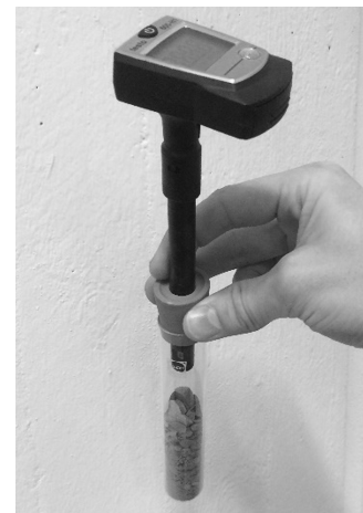
Figure 6- Capacitive RH-sensor (Testo 605-H1) attached on a test tube with a sample
