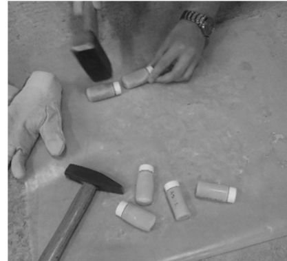
Figure 11 - Crushing samples with lump hammer.
