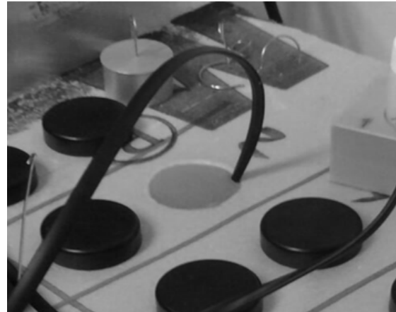
Figure 24 – Insulation sealing the space between hole and cable.
