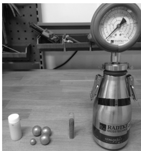
Figure 17 - Equipment for the carbide meter method.
