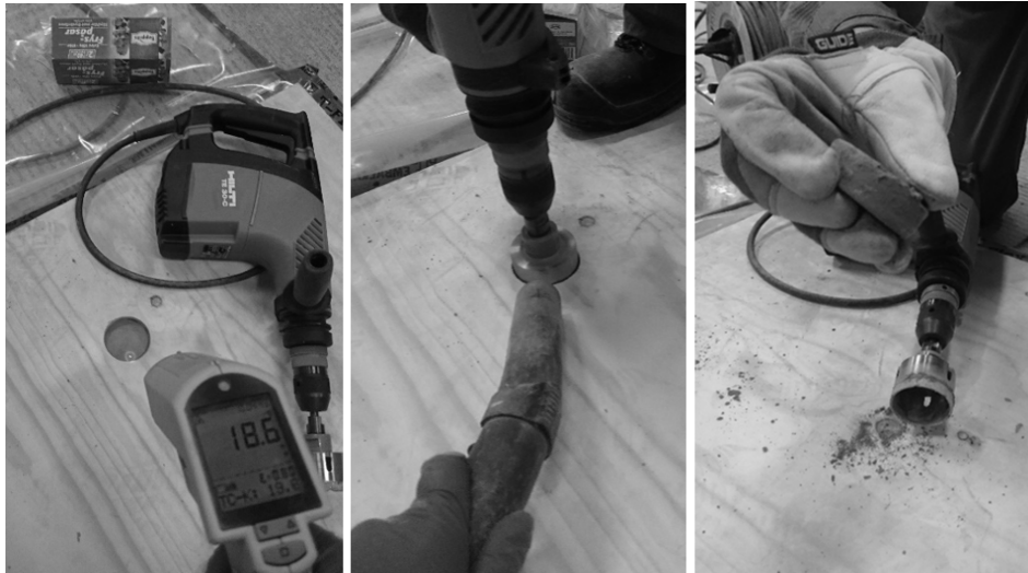
Figure 14 – From left to right: measuring of temperature with IR-thermometer, core drilling with vacuum cleaner and the SLC core after extraction.
