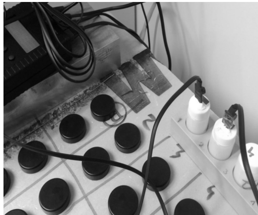
Figure 22 - Calibrating of RH-sensors with salt brines.
