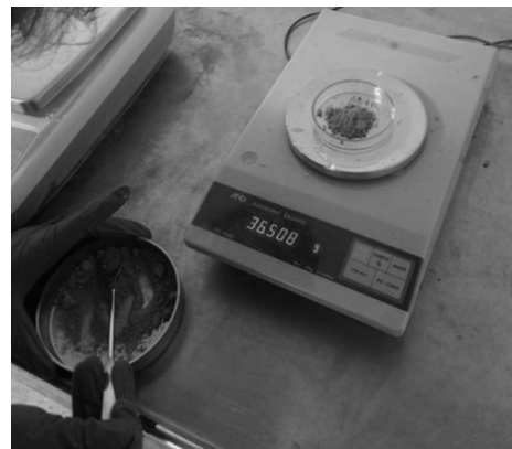
Figure 15 - Weighing of SLC before oven drying.
