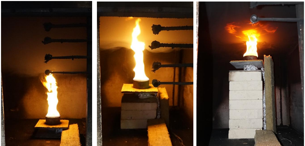
Figure 10. Photo made during the experiments depicting the flame – smoke layer interaction.
