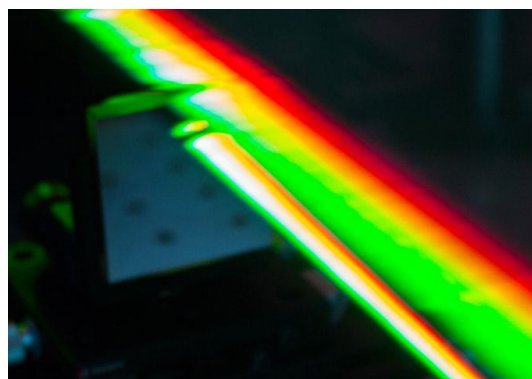
Figure 1: Spreading out the spectral components of short laser pulses makes it clear that the pulses contain light of different colors.
