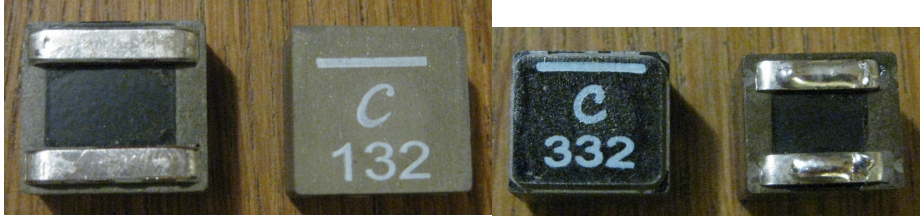
Figure 22: Coilcraft XAL1580(15.2 * 16.2 * 8 mm) and XAL1010 (10.0 * 11.3 * 10.0 mm)
